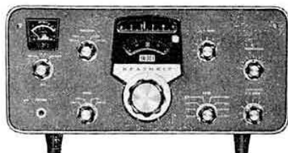
SB-301E Amateur Band Receiver . . . SSB, AM, CW and RTTY reception on 80 through 10 metres + 15 MHz WWV reception. Tunes 2 metres with SBA-300-4 plug-in converter. Kit SB-301E , 23 lbs. (less speaker) £125 Assembled £155
