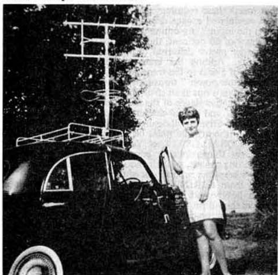
Path lengths up to 300 miles on 70cm were covered by GC8ARS/P from Jersey using this 8-over-8 slot array mounted on the vehicle roof rack. The lady is Mrs. G8ARS.
